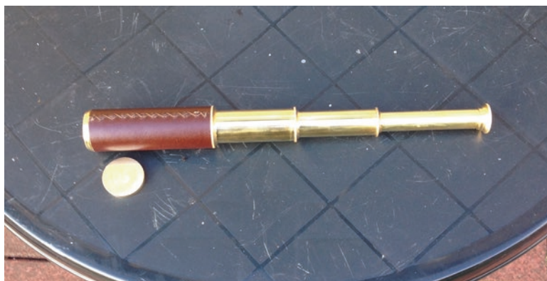
Fig. 1.3 The author's 6 \times achromatic spyglass used to corroborate Harriot's observations. (Image by the author)
