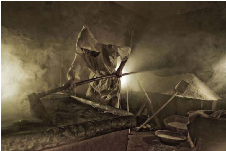
Fig. 2.1 Worker at a lead pan in a salt boiling house. Photographic reconstruction of the medieval working conditions (Photo provided by Lüneburg Marketing)
