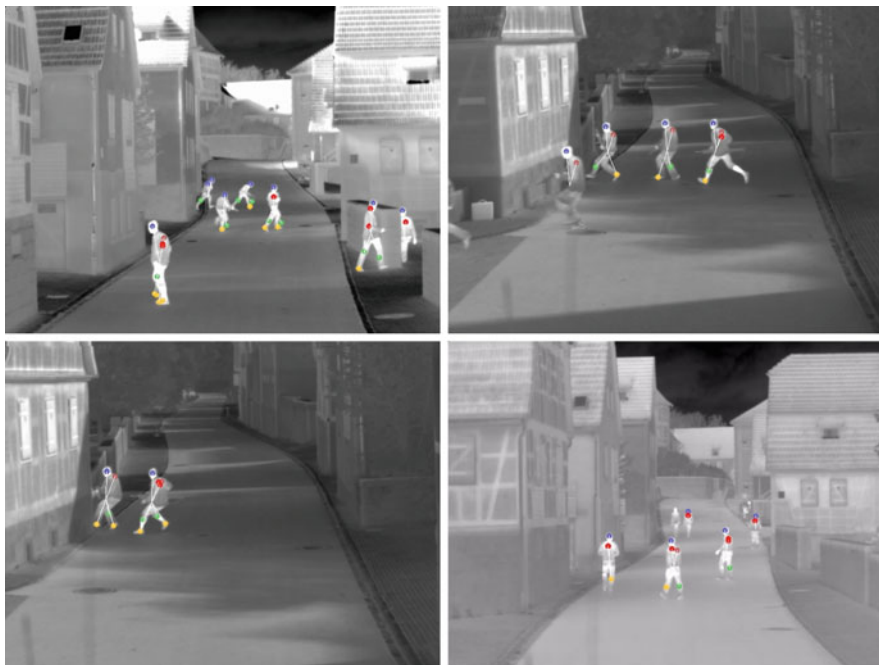
Fig. 3 Example body part classification results of detected persons. Relevant body part classes are: head, torso, shoulder, leg, and foot
