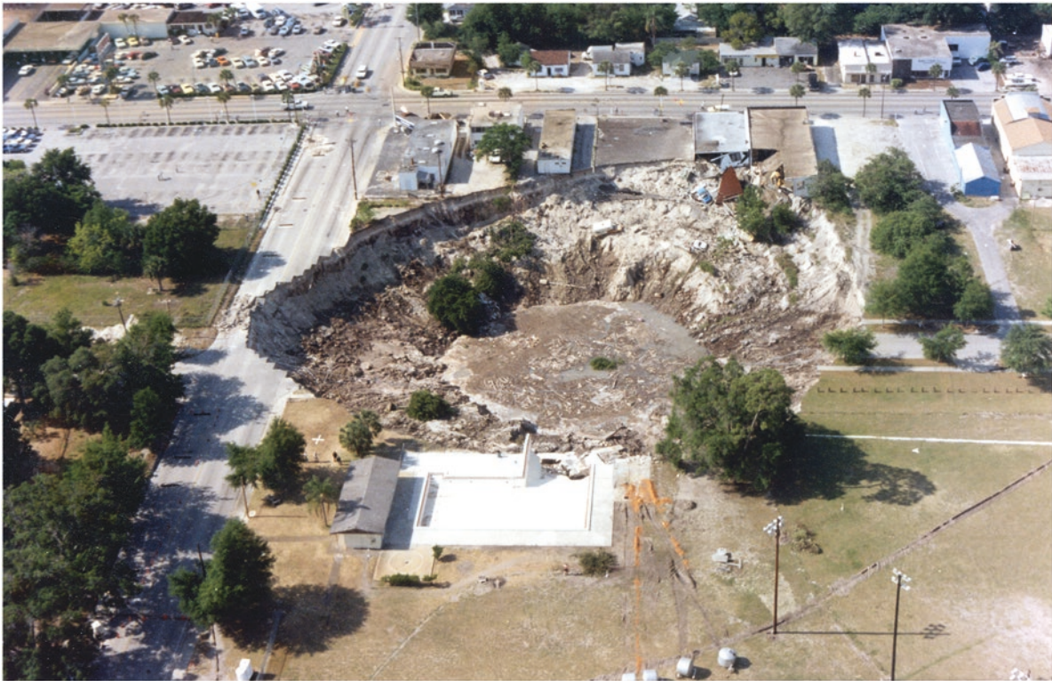
Fig. 1.5 The 1981 Winter Park sinkhole (28.594°N, 81.362°W), located in Winter Park, Orange County, Florida. The largest sinkhole
