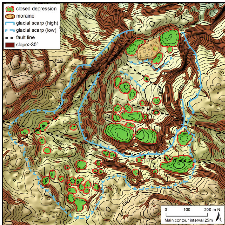
Fig. 1.4 GIS-based geomorphological map of a sample area in Canin Mountains (after Telbisz et al. 2011)
