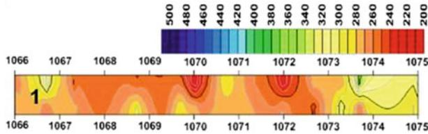
Fig. 4 Variation of stiffness measurements using kriging analysis
