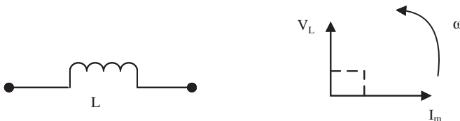
Figure 2.3 Phasor diagram of purely inductive circuit.
