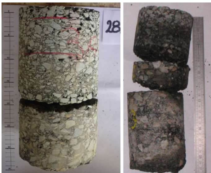
Fig. 1.1 Examples of cores from thick bituminous pavements, showing debonding of surface or internal layers
