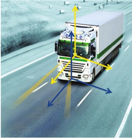
Fig. 1. Left: Different coordinate systems for cameras (LDW); yellow = camera coordinate system; blue = vehicle coordinate system Right: definition of the coordinate system
