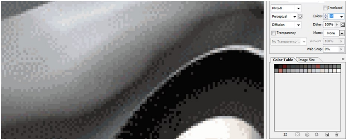
Figure 1-3. Showing the effect of dithering with an indexed color image compression setting of 32 colors (5-bit)
