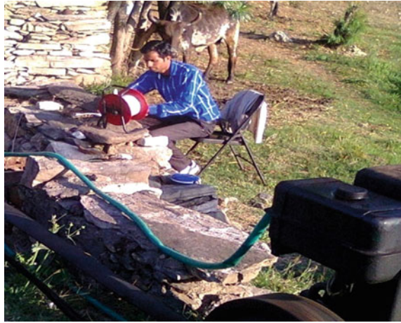
Fig. 3 Measurement of water level by using acoustic water level indicator
