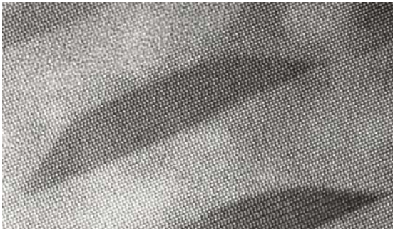
Fig. 1: HRTEM image of GaN quantum dots embedded in AlN taken along a \langle 2,-1,-1,0 \rangle direction
