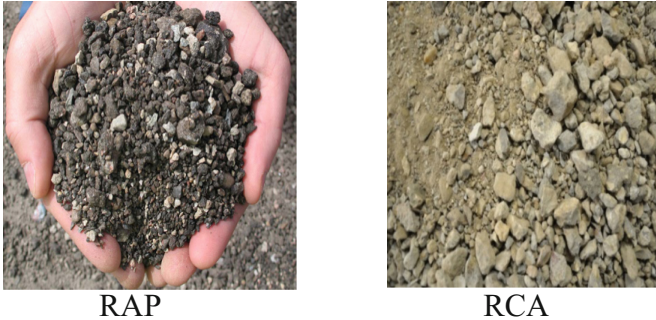
Fig. 1. Recycled asphalt pavement (RAP) and recycled concrete aggregate (RCA).
