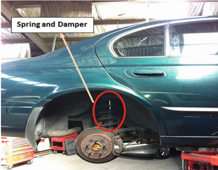
Fig. 1.1 Rear suspension system without wheel of a vehicle
