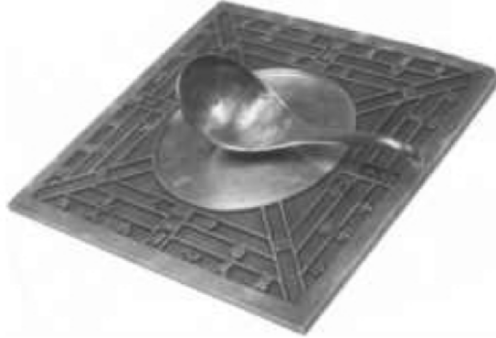
Fig. 1.2. Working model of the first instrument known to be a compass, called Si Nan (the south governor) by the Chinese. The spoon is of magnetic lodestone, and the plate is of bronze [10]
