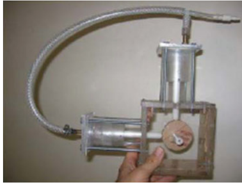
Figure 1.8 An Alpha Stirling engine.
